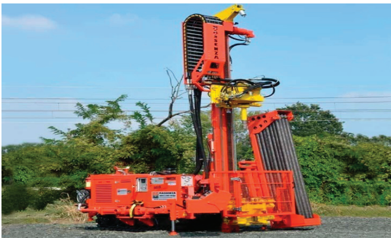
Fig. 4. Geothermal drilling rig deploying hybrid rotary-percussive technology (Source: Massena Drilling Rigs)
