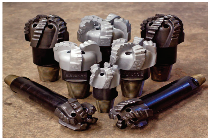
Fig. 3. Various PDC and hybrid drill bit configurations for hard rock applications (Source: Trenchless Technology)
