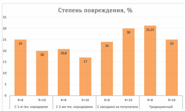
Fig. 3. Damage to soil, undergrowth and trees in technological areas, depending on the development scheme of the cutting area
